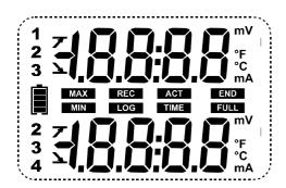
°C.....Temperature in degrees Celsius °F.....Temperature in degrees Fahrenheit V or mV....Voltage expressed in V or mV A or mA....Current expressed in A or mA END Data set is finished
